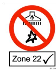
This standard covers the safety of dust extractors with electric motors, including dust separators and back-pack vacuums, used for wet extraction, dry extraction or wet-and-dry extraction, supplied for commercial use indoors and for outdoor use with and without accessories for the collection of combustible dust in an atmosphere (Zone 22) designated as explosive.
