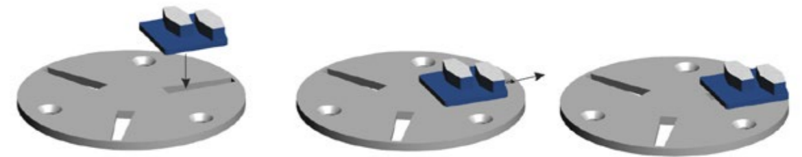
Figure 4-4 How to fit the diamond segments on the Scan-On plate
